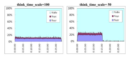
Figure 6-19 Comparison of CPU usage based on parameter value
