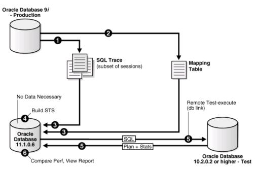
Figure 8-4 SQL performance test for upgrade from 9*i* to 10*g* R2
