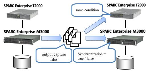
Figure 6-22 Overview of verification test
