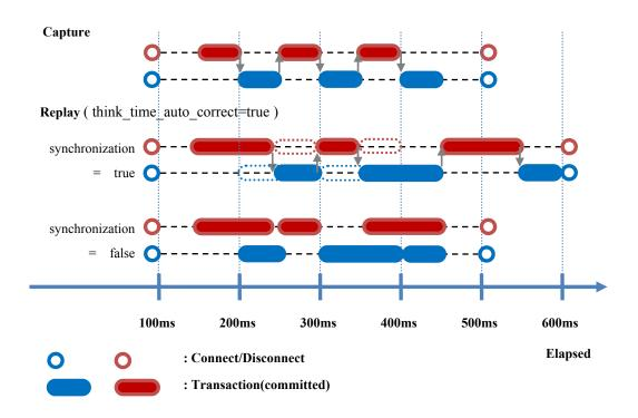
Figure 6-23 Effects of synchronization parameter
