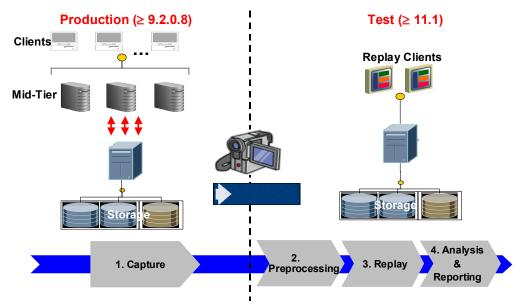
Figure 6-11 Main processing procedures of Database Replay
