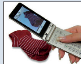
The photograph taken by the mobile-phone camera is used to display the name of the color.
