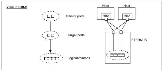
The SMI-S specification defines "view" as key concept to manage the masking and mapping function. The view consists of a set of the following items and represents logical volumes reported by SCSI REPORT LUNS command from any initiator port through any target port in the view.
