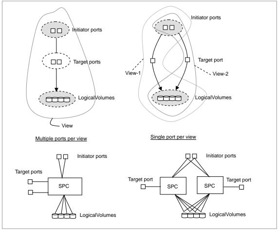
SMI-S sever implementation has an option for SPC –Single port per view. It means that a SPC can be related to only one target port. In single port per view, the view specified by ExposePath may be split into multiple views for each target port when multiple target ports are specified, and creates multiple SPCs.
