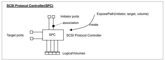
The method ExposePath is defined in SMI-S specification as a function to create view.
