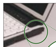
Connector cover (FMV-S8240) made from bio-plastic
