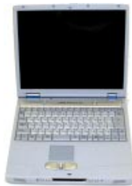
Prototype for a biodegradable plastic PC
