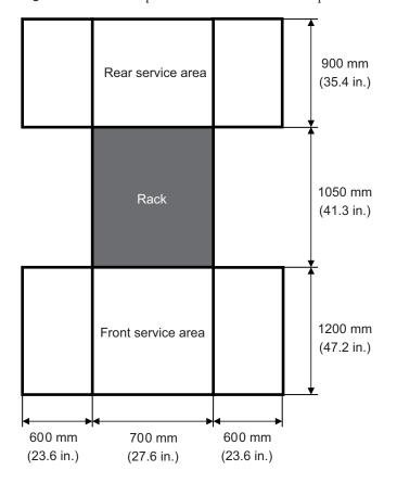
Figure 2-9 Example of service areas for an expansion rack (top view)
