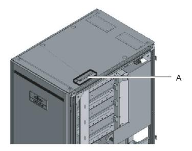
d. Insert the PDU connection side of the power cords through the top opening of the rack.
