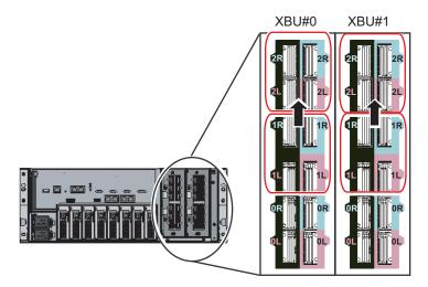
b. Replace the labels on the removed crossbar cables (optical).
