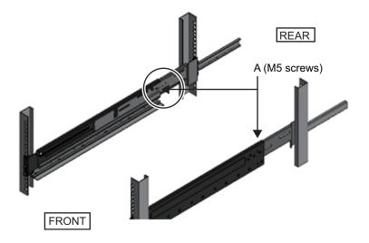
9. **Mount the chassis in the rack.** Mount the chassis from the front of the rack.
