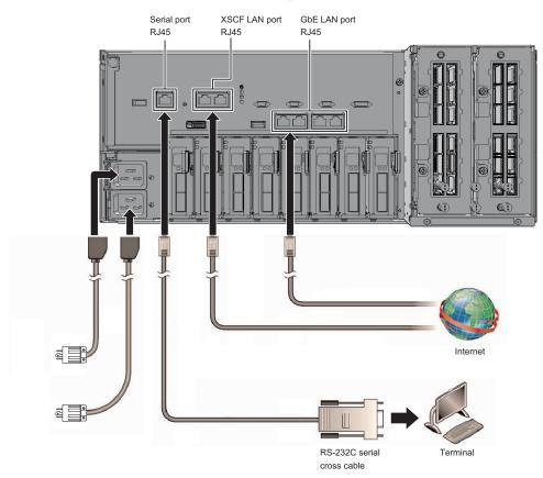
Figure 2-29 Network configuration example (crossbar box)
