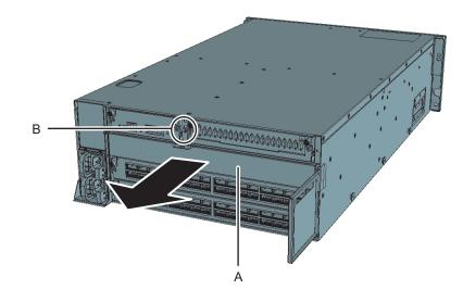
Figure 4-21 Removing the blank panel
