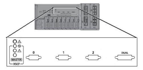
Figure 4-10 XSCF interface unit port locations (crossbar box side)
