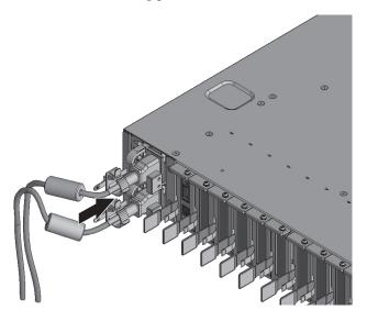
c. Secure the power cords with cable clamps. After locking each clasp (A in Figure 5-14), push the cable clamp toward the front of the chassis to firmly secure the clamp.
