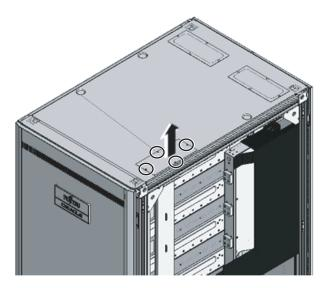
c. Fit the protection bushing (A in Figure 3-6) in the top opening of the rack.
