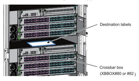
Figure 5-4 Destination label storage location: Top panel of the lower crossbar box
