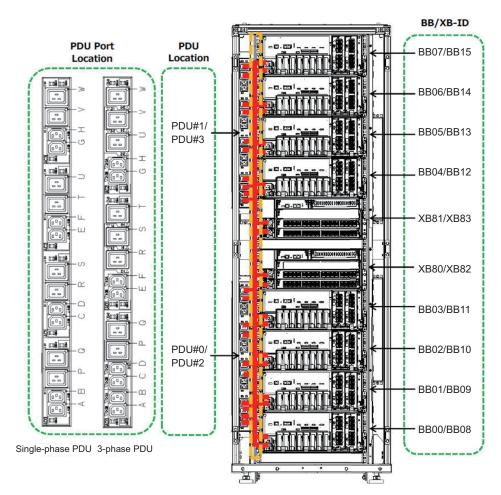
Figure 5-20 Power cord wiring diagram
