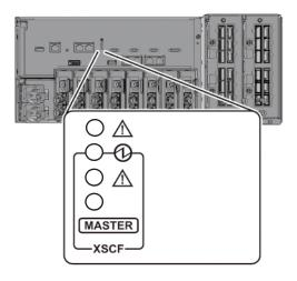
Figure 6-4 Rear view of a crossbar box
