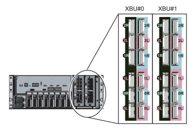
Figure 4-6 Example of the appearance of a crossbar cable label
