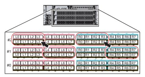
Figure 4-23 Moving cables of XBBOX#80/#81
