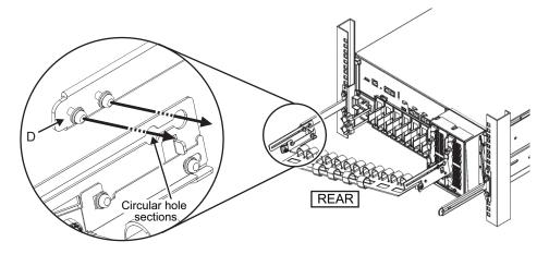
b. Slide in the cable support all the way, and tighten the four screws (C in Figure 3-47).
