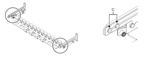
b. Slide the cable support fixing brackets (D in Figure 3-69) to remove them.
