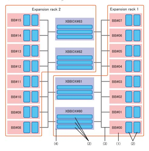
Figure 1-2 Connections through crossbar boxes
