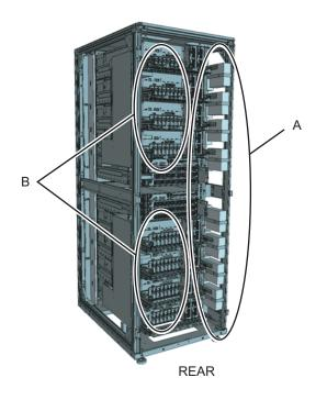
2. Pass the crossbar cables (optical) unwrapped in step 1 between the upper and lower PDUs on the connecting part of the racks.
