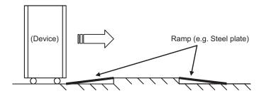
• Since the maximum weight of an expansion rack may be about 960 kg when packed and 780 kg when unpacked, confirm in advance that the access route has no problem with that weight.
