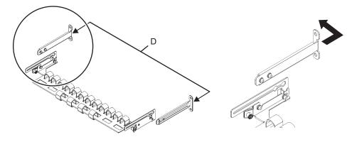
c. From the rear of the rack, secure the rails and cable support fixing brackets (D) with two M6 screws to the rear supporting columns of the rack. The fixing locations are 1U center and 2U center.
