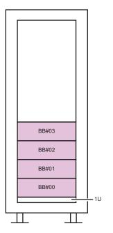
**Note** - For SPARC M10-4S maintenance, the cable support at the chassis rear moves underneath the chassis, so do not mount anything in the lowest shelf (1U) of the rack.
