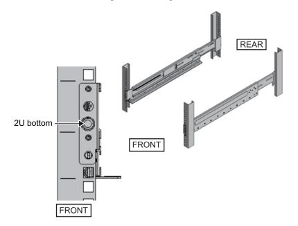
Attach the cable support fixing brackets to the rear supporting columns of the rack.
