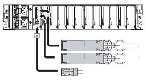
Figure 5-10 Connecting the link cables and management cable (SPARC M10-4S side)
