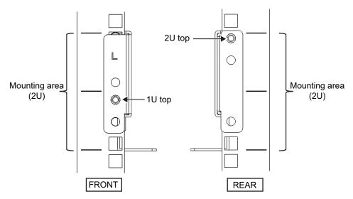
Figure 3-64Attaching the Type-2 rail: Fixing location of the screw (for<br/>supporting columns having square holes)
