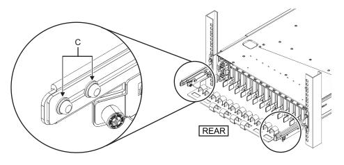
Figure 3-78Attaching the cable support (2)
