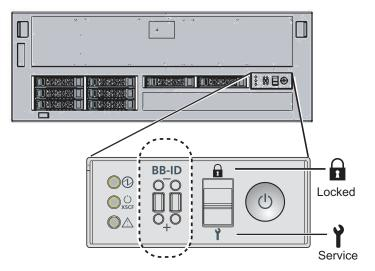
Figure 6-2 Mode switch on the operation panel of a crossbar box
