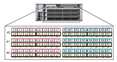
Figure 4-19 Example of the appearance of a crossbar cable label
