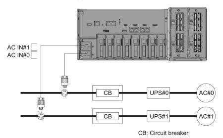
Figure 2-21 Power supply system with UPS connections
