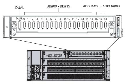
Figure 4-11 Example of the appearance of an XSCF cable label (SPARC M10-4S side)
