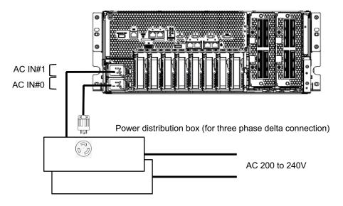
Figure 2-19 Power supply system with three-phase power feed (expansion rack: single power feed)
