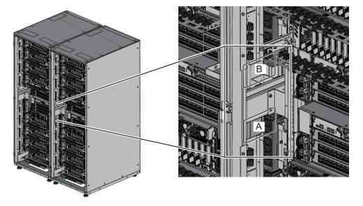
Figure 4-14 Locations for passing cables between the racks
