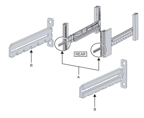
Figure 3-66 Attaching the cable support fixing bracket
