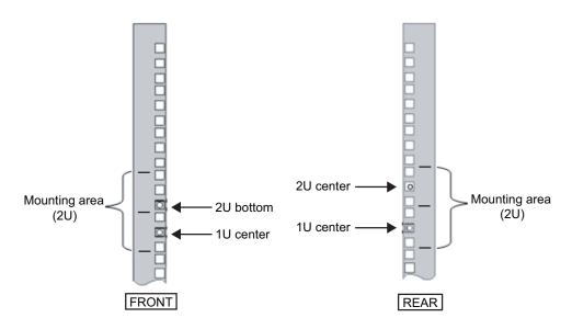
a. Attach cage nuts from the inside of the rack.
