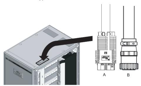
e. Connect the power cords to the PDUs. Each cable has an attached label showing the connection destination. Each PDU also has an indicator. So, match it with the right cable to connect the cable. For the PDU mounting locations, see Figure 3-8.
