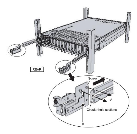
Figure 3-76 Attaching the cable support
