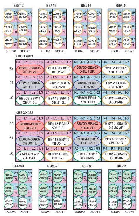
**Note** - The colored areas in the diagram indicate the cables that pass between the racks. See the correspondence tables in Table B-13 and Table B-14.
