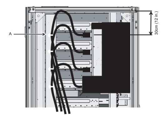
**Remarks -** Figure 3-13 shows single-phase power feed. The required lengths are the same as for three-phase power feed.
