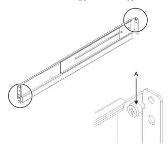
4. **Remove each screw from the side of the rail.** For the Type-1 rail, remove the one screw (A in Figure 3-60) from the side of the rail.
