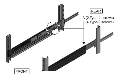
8. **Mount the PCI expansion unit in the rack.** Mount the chassis from the front of the rack.
