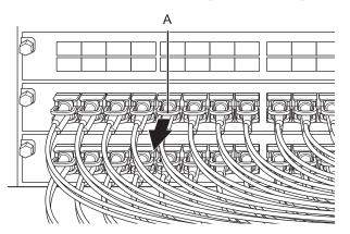
b. Replace the labels on the removed crossbar cables (optical). The replacement labels are supplied with expansion rack 2. Referring to Table 4-1, replace the labels.
