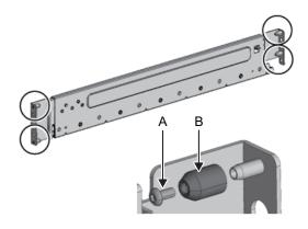
5. **Remove the one screw (A in Figure 3-32) from the side of the rail.** The removed screw will be used in step 8.
