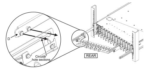
b. Slide in the cable support all the way, and tighten the four screws (C in Figure 3-78).
