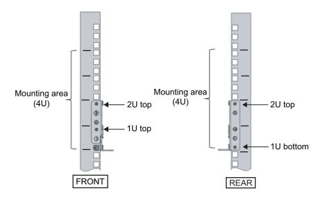
Figure 3-34 Attaching the rail: Fixing location of the screw
