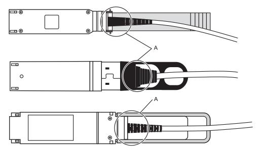
Figure 4-27 Part to hold when checking a crossbar cable (optical) connection
