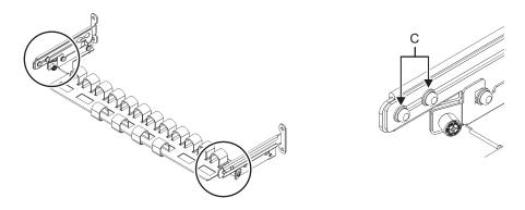
b. Slide the cable support fixing brackets (D in Figure 3-38) to remove them.
