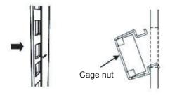
b. Insert the hook at the tip of the supplied cage nut attachment tool through a cage nut attachment hole from the front, and engage it with the hook at the other end of the cage nut.
