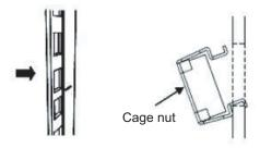
b. Insert the hook at the tip of the supplied cage nut attachment tool through a cage nut attachment hole from the front, and engage it with the hook at the other end of the cage nut.
