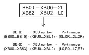
**Note -** The label shows both the cable connection destination and the unit connected by the cable.
