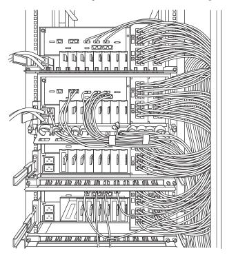
Figure 5-17 Example of stored cables (4BB configuration)
