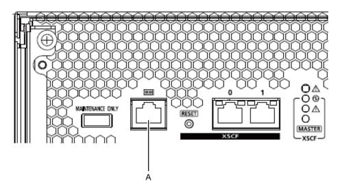
2. Connect a LAN cable of Category 5 or higher from a GbE port (A in Figure 5-2) to the network switch or hub.
