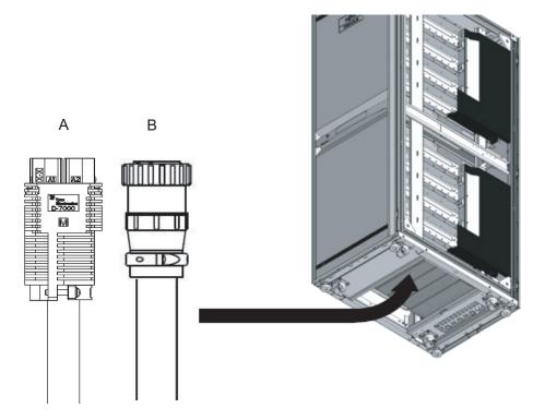
c. Connect the power cords to the PDUs. Each cable has an attached label showing the connection destination. Each PDU also has an indicator. So, match it with the right cable to connect the cable. For the PDU mounting locations, see Figure 3-12.
