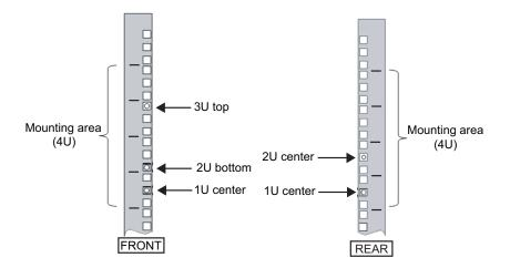
a. Attach cage nuts from the inside of the rack.Orient the hooks of the cage nut vertically.Hook the hook at one end of a cage nut into a cage nut attachment hole of the rack.
