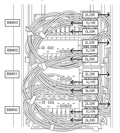
Figure 5-18 Example of stored cables (4BB configuration)
