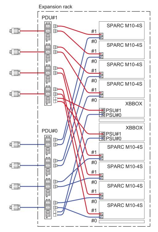
Figure 2-23 Power supply connections for an expansion rack (three-phase delta connection/three-phase star connection)
