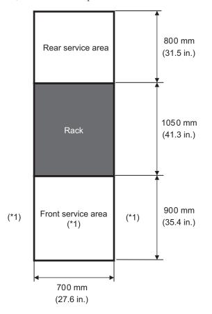
\*1 To mount a chassis on the rack, an area with a depth of 1,200 mm (47.2 in.) is required in front of the rack, and areas with a width of 600 mm (23.6 in.) are required on both the left and right sides of the front service area. If there is a possibility that a chassis will be added later, secure an area with a depth of 1,200 mm (47.2 in.) in front of the rack and areas with a width of 600 mm (23.6 in.) on both the left and right sides of the front service area.
