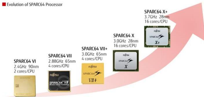
Fujitsu processor design team has been working on performance and reliability improvements and innovations over many years. The SPARC64 X and SPARC64 X+ processors used in the Fujitsu M10 represent the leading edge of this process.
