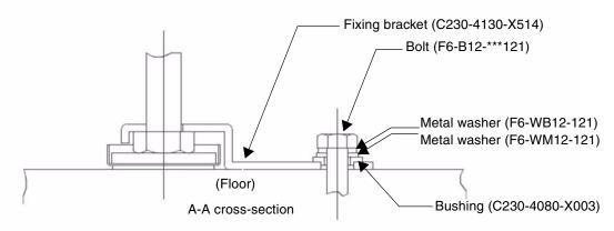
FIGURE 6-2 Example of Securing the Cabinet Through a Hole in the Floor
