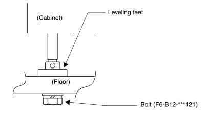
FIGURE 6-2 Example of Securing the Cabinet Through a Hole in the Floor
