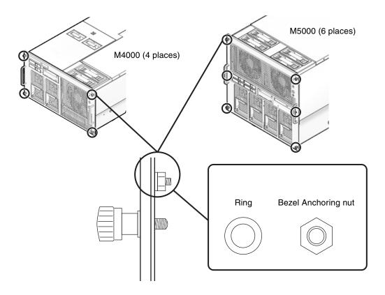
2. In place of the removed nut and ring, attach the E-Ring, included in the rack mount kit.
