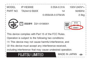
Figure 2-2 Label at the bottom of the IP-HE900E (e.g.)
