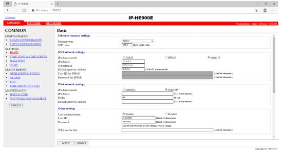
Figure 3-2 Screen for IP-HE900 DECODER Settings
