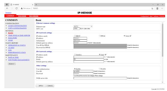
Figure 3-1 Screen for IP-HE900 ENCODER Settings
