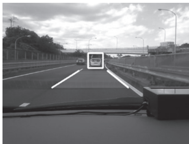
Figure 4 Smartphone camera image for detecting road marker lines and vehicle in front.
