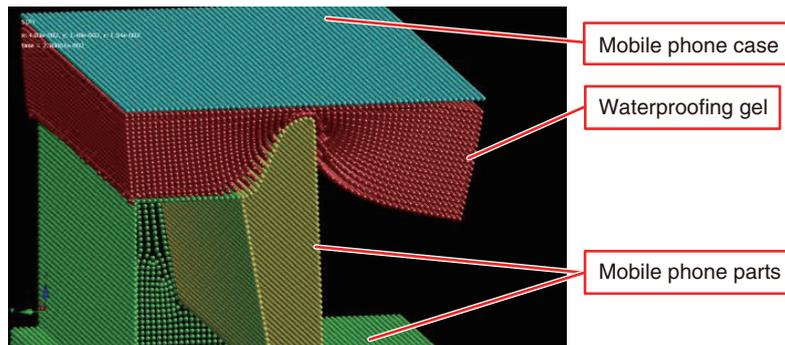
(b) Large deformation analysis of waterproofing gel used in mobile phones
