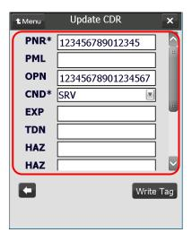
(2) Click the **Write Tag** button to write the Current Data Record that has been entered to the tag.
