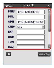
(2) Click the **Write Tag** button to write the Lifecycle Record that has been entered to the tag. Clicking the Back button returns to the previous screen.
