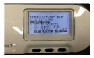
(8) Press the **DOWN** button until the **SET IP ADDRESS** is highlighted, then press the **SELECT** button
