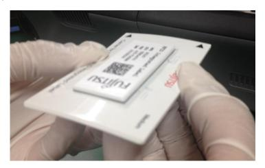
Bend down the carrier holding both longer sides to opposite direction against the carrier facing up label surface.
