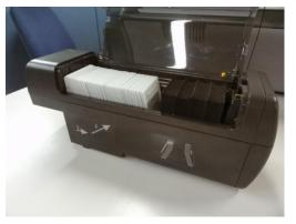
! Caution The Shock Absorber MUST be placed between the stack and the Card Stack Pusher
