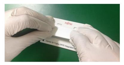
Press the RFID Label against the notch of the Reusable Carrier.
