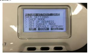
(5) Press the **DOWN** button until the **DHCP MODE** is highlighted, then press the **SELECT** button
