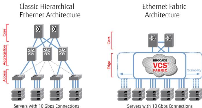
Figure 1: Compared to classic Ethernet architectures, Ethernet fabrics allow all paths to be active and provide greater scalability—while reducing management complexity.
