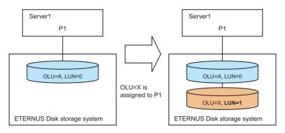
When OLU=A has been assigned to P1 as LUN 0, LUN 1 assigned to OLU=X when OLU=X is assigned to P1.
