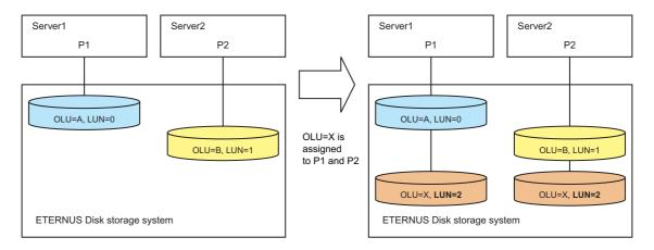
When OLU=A has been assigned to P1 as LUN 0 and OLU=B to P2 as LUN 1, LUN 2 is assigned to OLU=X when OLU=X is assigned to P1 and P2.
