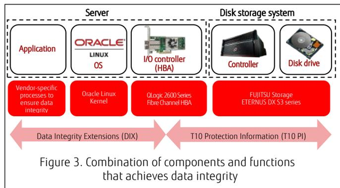
Figure 3. Combination of components and functions that achieves data integrity
