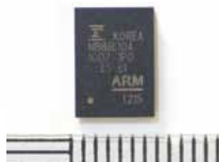
RF transceiver LSI for mobile phones compatible with LTE, a next-generation communications format
