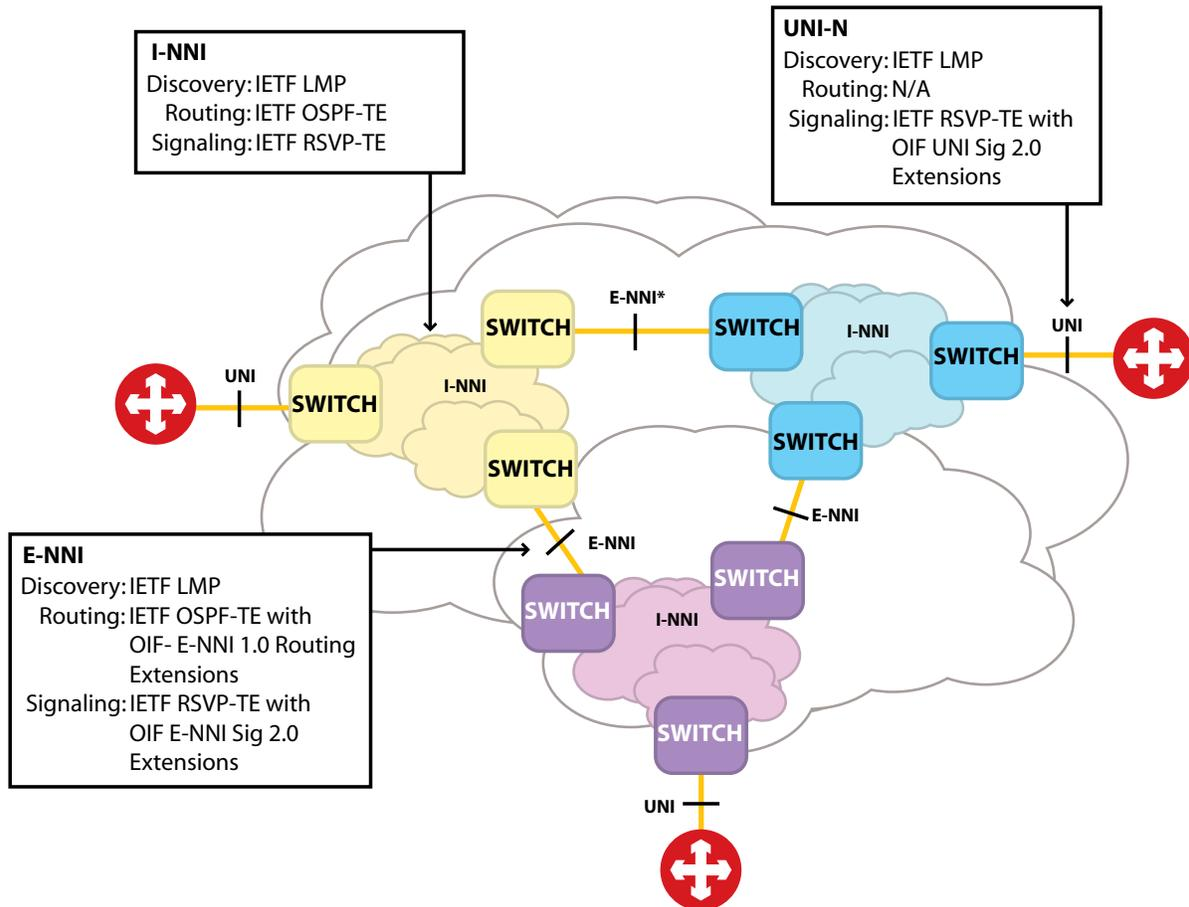
**Figure 12: The Fujitsu Control Plane Approach**
