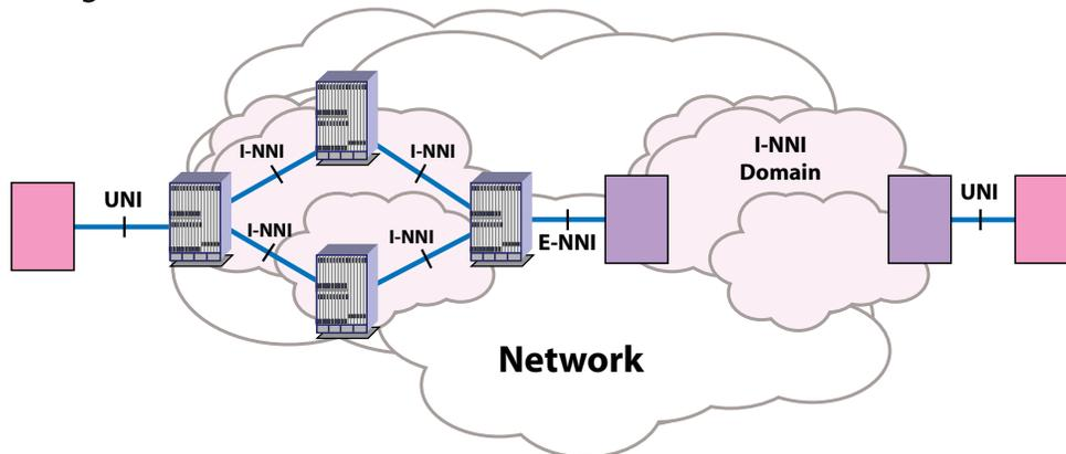
**Figure 4: ITU-T Network Reference Points**
