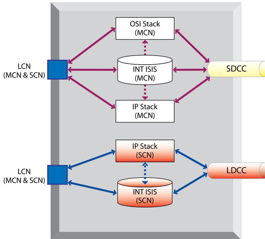
**Figure 15: MCN/SCN Separated Operating Mode**
