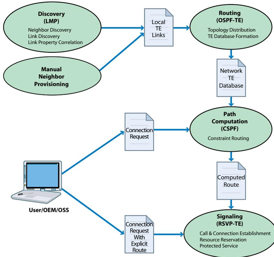
**Figure 11: Control Plane Application Interaction**
