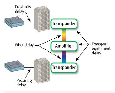
Figure 1: Sources of latency in optical transport networks
