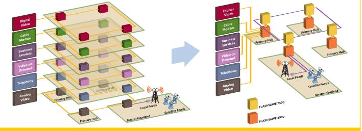
Progression from Overlay Networks to a Multiservice Network with the FLASHWAVE 7500 Platform
