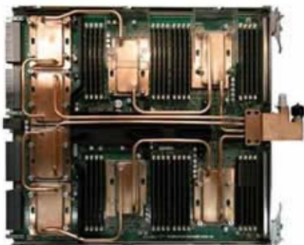
Figure 1 Cooling water piping on PRIMEHPC FX10 system board
