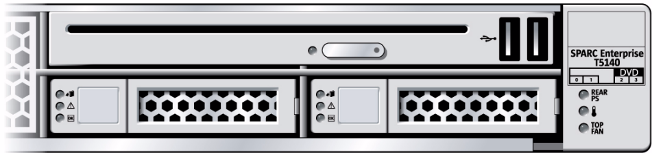
FIGURE: DVD/USB Module in a SPARC Enterprise T5140 Server
