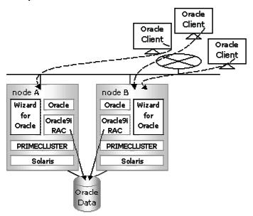
In scalable operation with Oracle9i RAC, Oracle is operated on all nodes. Regardless of which node a client is connected to, the client is able to use the database.
