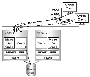
In standby operation, a cluster system consists of an operational node and standby nodes. On the operational node, Oracle applications, a logical IP address and shared disks are active. On the standby nodes, these resources are inactive. In the event of a failure, business operation is switched to one of the standby nodes, and the resources in this standby node are activated. Then, the client can be connected to the running node using the logical IP address without modifying any settings.
