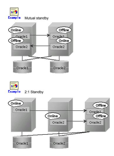
On the standby nodes, the database on the shared disk created from the operational node should be enabled. This is the same as other operation methods.
