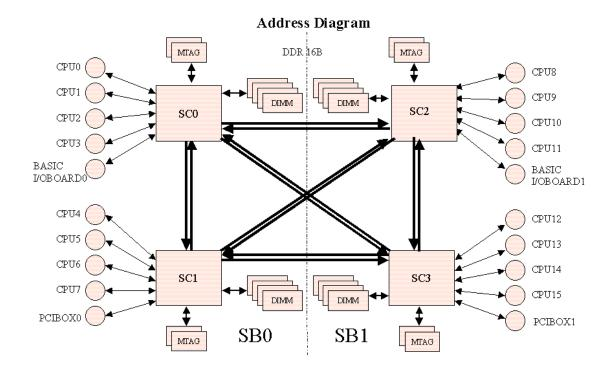
As shown in the figure below, the data system is divided into four groups. Each group connects with four CPUs and an I/O bridge.
