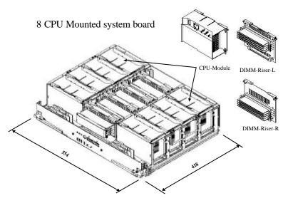
To increase the mounting density, eight CPUs are mounted on one system board. In addition, to fully utilize the space, the DIMMs are mounted three dimensionally using a riser card. 32 GB of memory can be mounted per system board. The DDCON section of the power supply has also been decentralized and mounted on the system board and CPU modules. The result is that mounting density of the power supply has been greatly increased.
