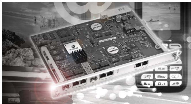
The reference board featuring Fujitsu's MB87M2181 and Switchcore CXE2139 devices: a compact solution for service aware Ethernet over SDH/SONET applications.
