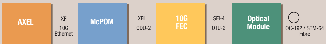
Fig 4: McPOM used together with 10G Ethernet switch
