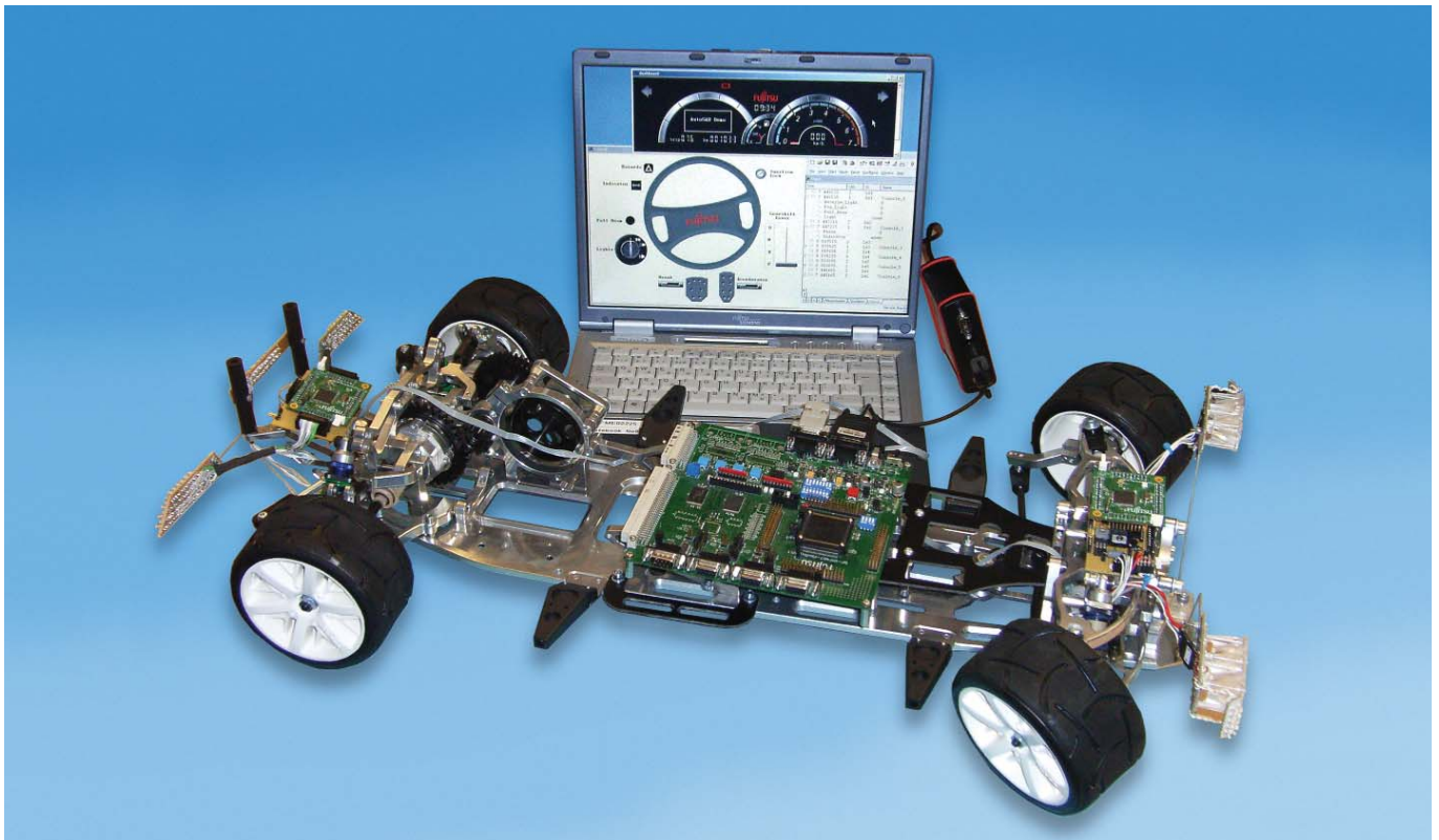
AUTOSAR Roadster featuring Fujitsu's 32-bit microcontrollers series MB91460 operated by application and basic software modules compliant to AUTOSAR 2.0.
