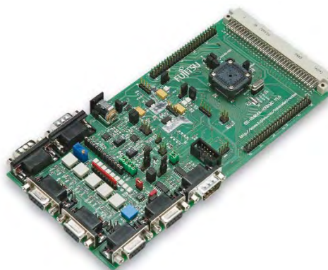
SK-91F465X-100PMC evaluation board.
