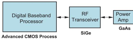
Figure 2 – Block Diagram of an RF System
