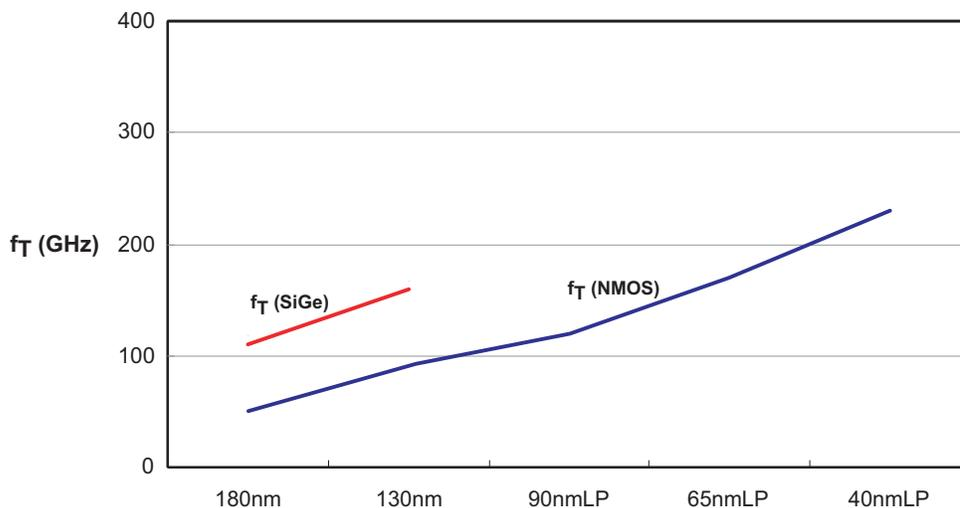
Figure 4 – Typical  $f_T$  for NMOS and BJT Transistors in CMOS and SiGe Processes, Respectively (GHz)
