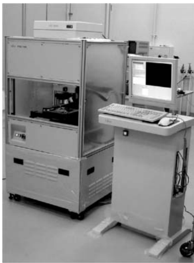
Figure 14 Light-guiding plate and metal mold measurement system.
