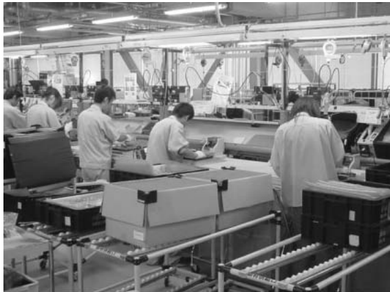
(a) Supplying parts from the side (before improvement)
