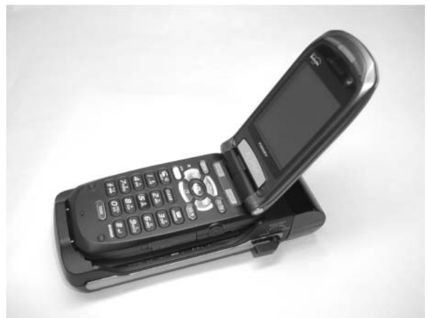
Figure 10 Mobile phone mounted on newly developed \mu -FC module (cradle type interconnection).
