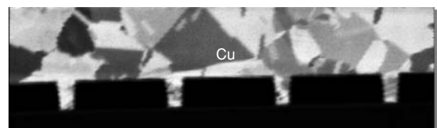
(c) 11 days after ECD-Cu (grain size > 1 \mu\text{m} )
