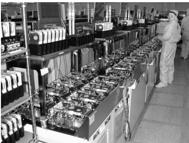
Figure 1 Servo track writers in a product line.
