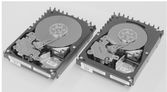
Figure 4 10 krpm AL-7LE (left) and 15 krpm AL-7LX (right).
