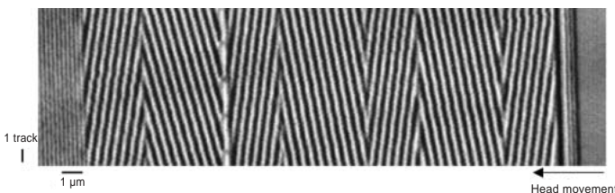
Figure 14 MFM photograph of position signal on AL-7LE media.
