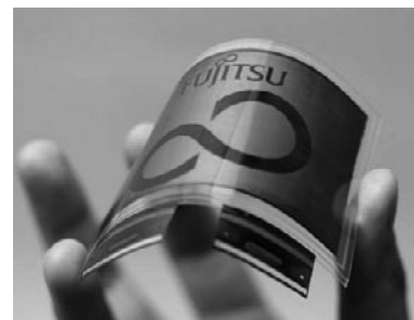
3.8-inch display area, mono-color type electronic paper (Announced July 2005)
