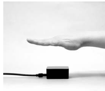
Fig. 4. Palm vein sensor
