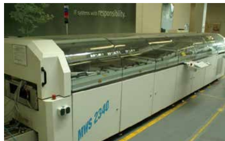
Flow soldering equipment using low-temperature solder
