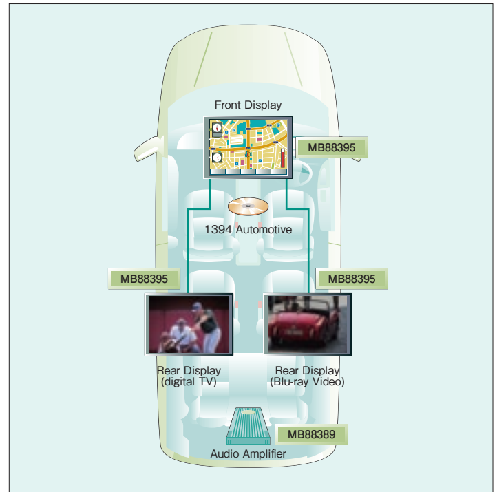
Figure 1 Application Image for 1394 Automotive in a Car
