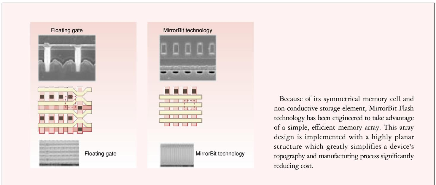
Because of its symmetrical memory cell and non-conductive storage element, MirrorBit Flash technology has been engineered to take advantage of a simple, efficient memory array. This array design is implemented with a highly planar structure which greatly simplifies a device's topography and manufacturing process significantly reducing cost.
