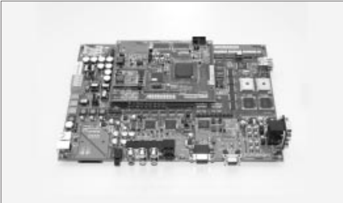
Photo 2 CPU subboard and SoC baseboard
