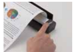
The page is scanned. Press the scan button to end the scanning process and create the PDF image file.
