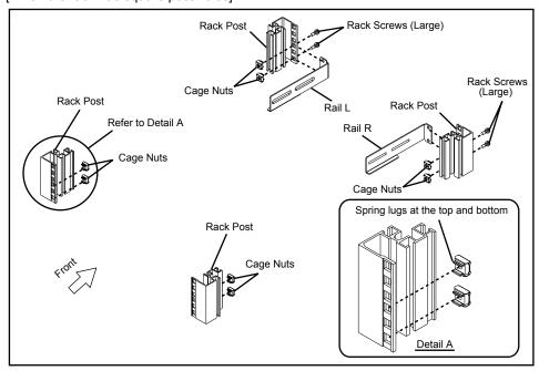
[When the rack has round post holes (top of view)]
