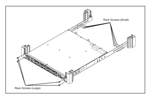
2. Slide the XG2000C forward, and remove it from the rack.
