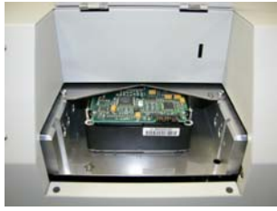
Second pass, PCBA faces up (Universal Attachment is not used).
