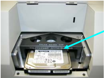
First Pass with PCBA facing down
