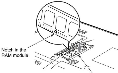
**6 Attach the expansion RAM module slot cover as it was.**
