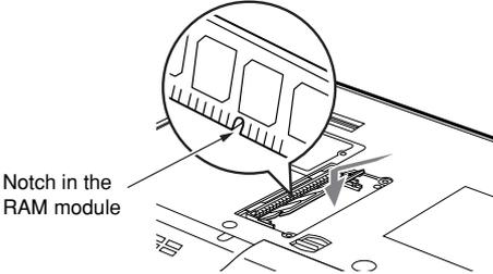
Check to see that the memory is fastened securely by the tabs on both sides. If a tab is in a state shown below, the memory is not mounted correctly.
