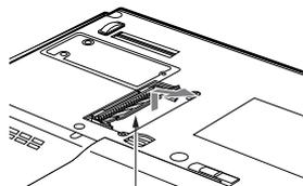
Expanded RAM module slot (DIMM1)
