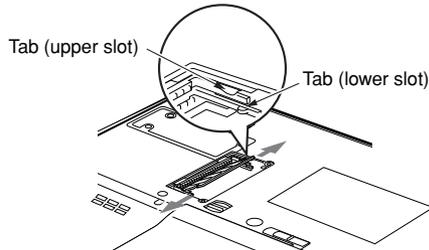
2. Similarly, open the tabs on both sides of the upper slot. This causes the memory to come up further.
