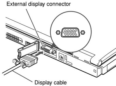
**3 Connect the display cable to the CRT display.**
