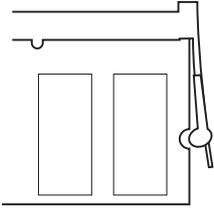
In this case, further push the memory into the slot.
