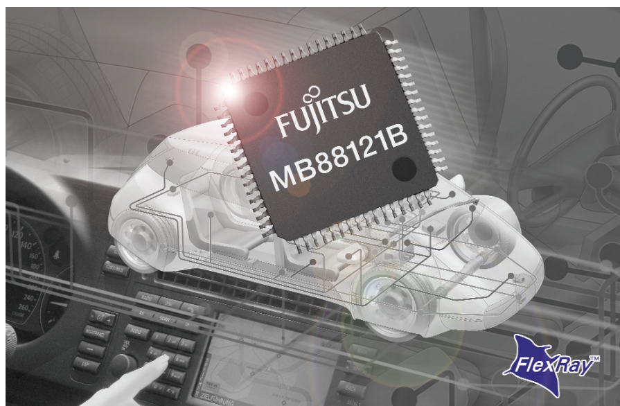
MB88121B adds FlexRay connectivity to 16-bit and 32-bit microcontrollers that lack embedded FlexRay protocol engines.
