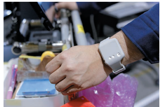
Vital-sign sensing band attached to worker's wrist
