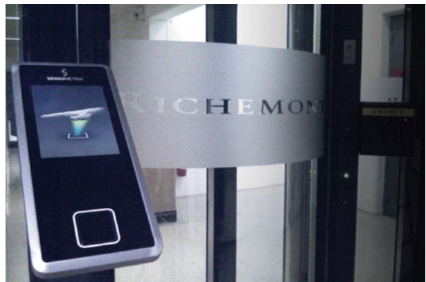
Security access system using PalmSecure™ palm vein authentication
